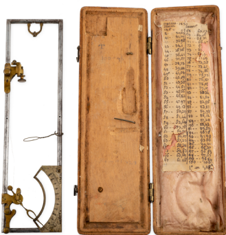
The hair hygrometer, invented by Horace Bénédict de Saussure.
